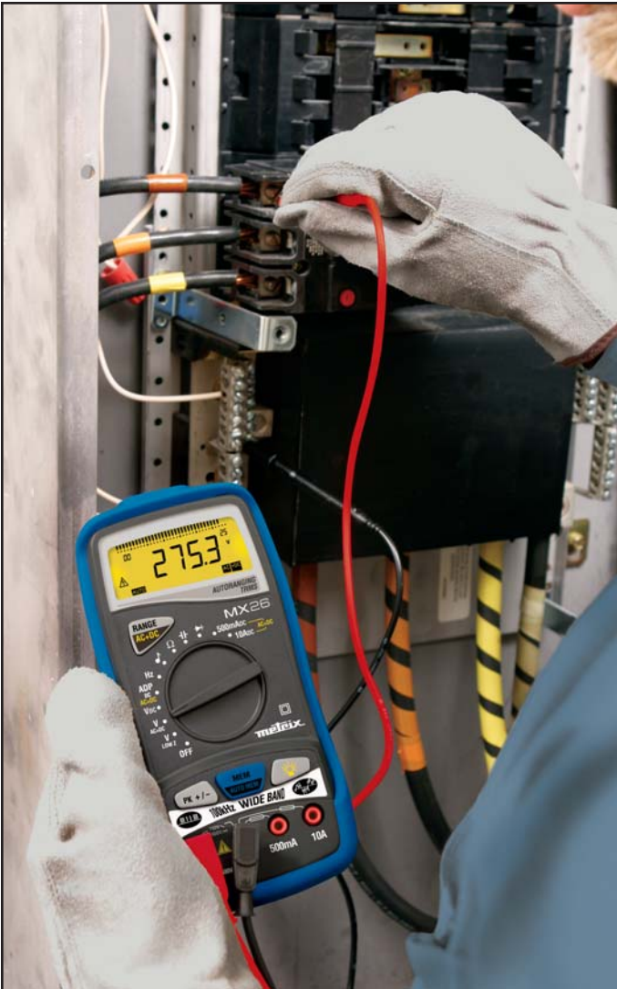
Model MX26 measuring feeder voltage on a 3-phase panel
