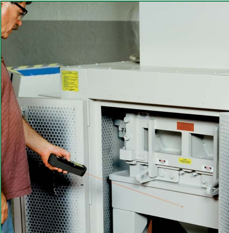
Laser guide allows you to take accurate and safe temperature measurements on extremely hot surfaces.
